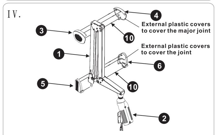
Take three pcs of pin to press and fix the external plastic covers according to the location, that shown from the drawing.
