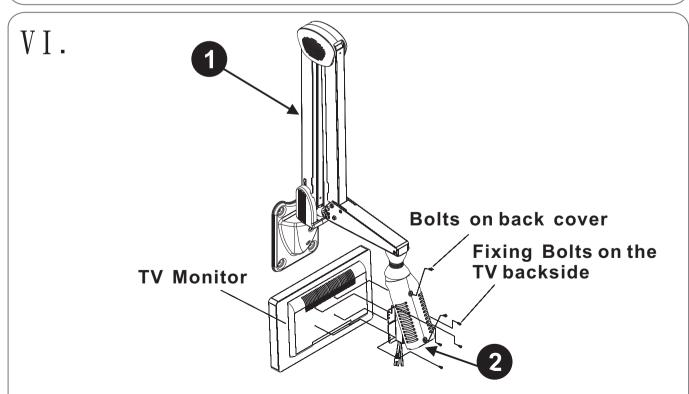
Use four Bolts to fix the TV monitor, then use two Bolts to fix the back covers. Connect the electric wire with the slot.
