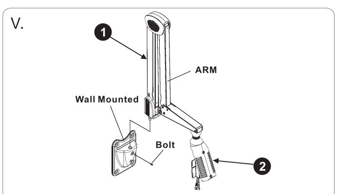
Plug in the main arm in the slot at the wall mounted, Use the fixing Bolts to lock according to the attached picture.
