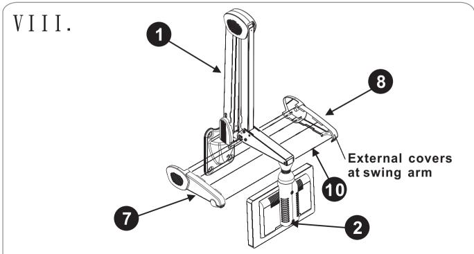
Take five pcs each of pin and swing arm external covers push, Press to the fix feature according to the location shown from the picture.
