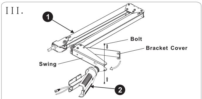
Once the electric wire is in the right position, then cover the bracket cover and use the bolt to tighten the two sides of the main swing arm.
