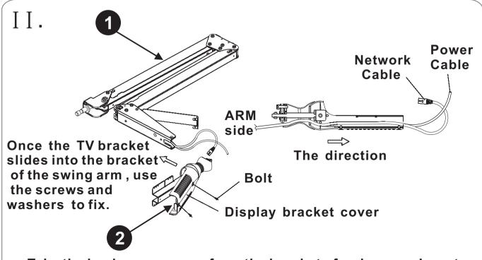
Take the back cover screw from the bracket of swing arm, Insert the electric wires according to the attached photo, Use the Bolts and washers to fix.
