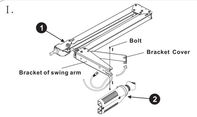
Remove the screws from the swing arm covers, and lift the bracket cover at the main arm.
